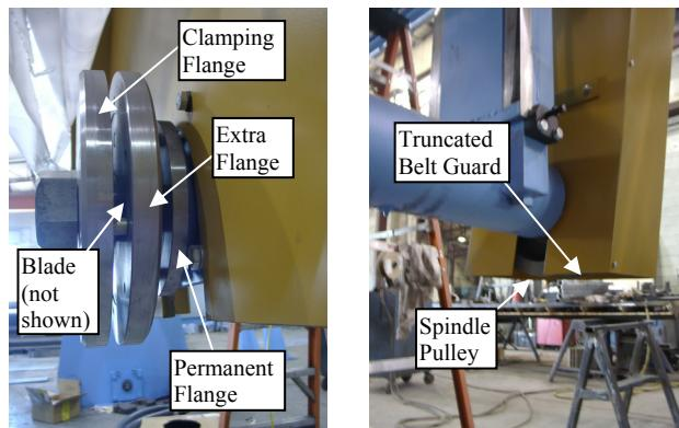
Saws with arbor motors don't have spindle pulleys but then the motor diameter limits the depth the same way. Spindles with drive pulleys can be made smaller in diameter than an arbor motor for the same horsepower and speed.
