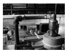
Side view of hose assembly as installed. The A-4175-60 repair kit consists of two 3/8" male hose adapters, 6" of 3/8" rubber water hose, and two 3/4" O.D. hose clamps.
