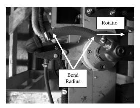
Turn elbow and install 3/8" hose assembly with approximate bend as shown looking down from above machine. (Rotation of spindle is clockwise from above.) Cut hose to required length to achieve bend (approx 5.25", but check before cutting.) Use pipe sealant on threads of hose adapters.
